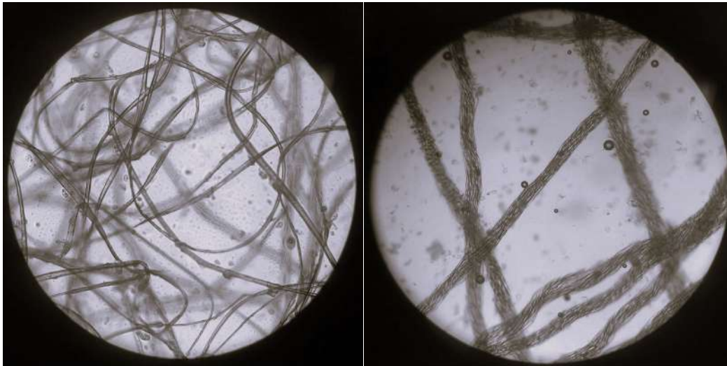
Photo.6,7. Microscope photo of raw silk (left) and silk fibers (right) 2021 source: author's archive
