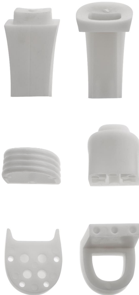
Figure 79. Heels created for the purpose of this research work, printed on a 3D printer
