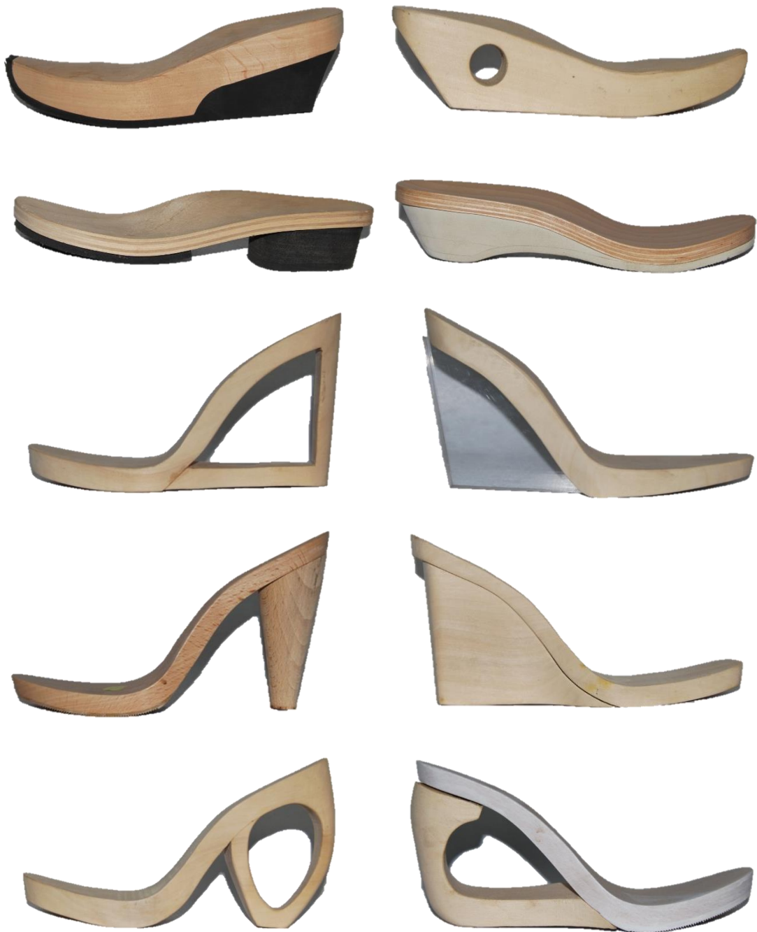
Figures from 52 to 61 – various forms of heel forms for the same form of shoe bottoms. From the author's own archive
