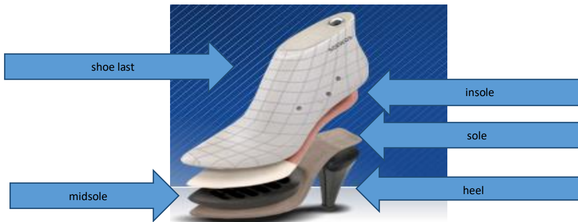
Figure 45. Components of footwear
